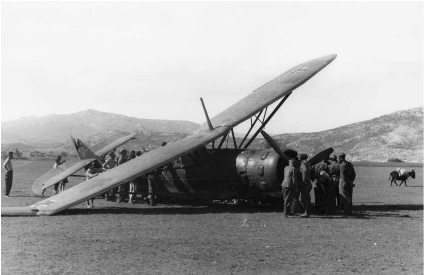
Minutes later, the take-off run of the Hs 126B-2 ended with a crash. The most common cause of such accidents was a swerve during the run, either due to pilot error or strong winds, and overwhelming pressure leading to break-up of one of the landing gear legs.
