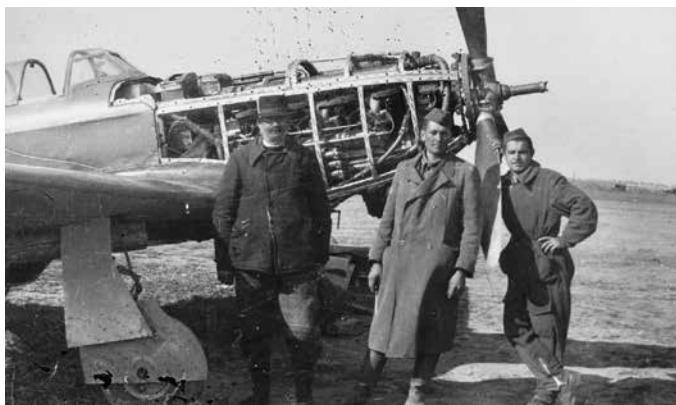
Mechanics working on the 1.210 HP Klimov VK-105PF engine of a TLK Yak 1b.
