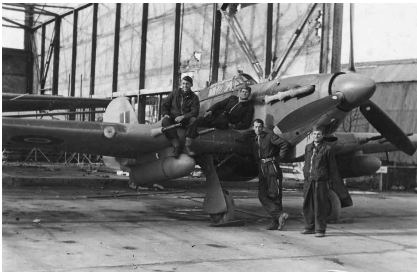
Members of Liaison Escadrille VŠ NOVJ with Wing Commander Selby's Hurricane Mk.IV at Zemun aerodrome in February 1945. The aircraft carries two 44 gallon auxiliary drop tanks. Seen behind is the left wing tip of the trophy Ju 52, which was captured by Partisans at Kapino Polje on 4 November 1944.
