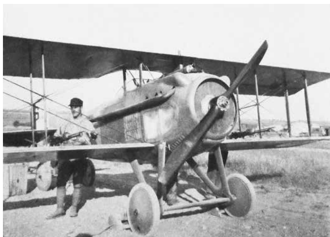
One of just two SPAD VII C1 fighters armed with three machineguns known to have served on the Salonika front.
