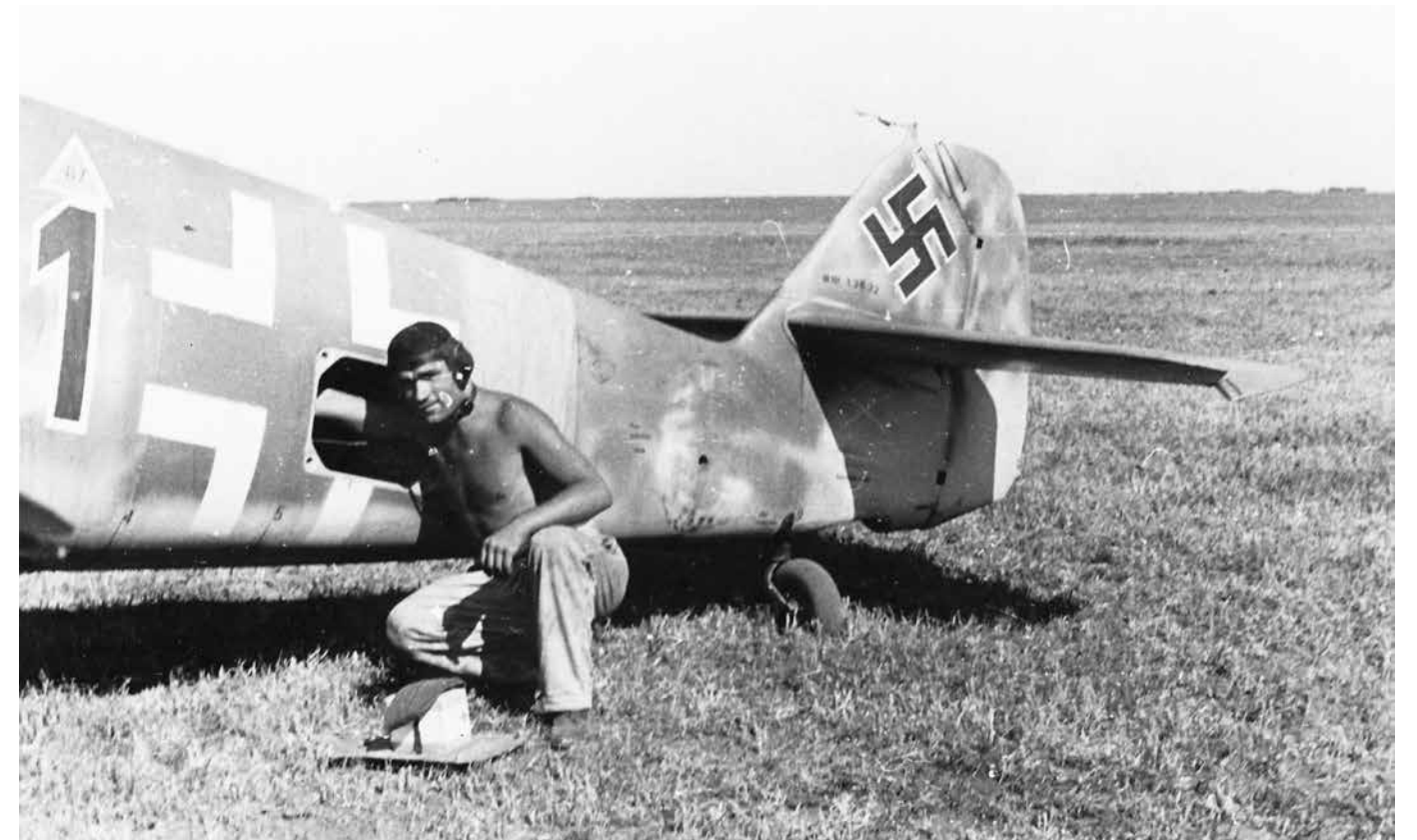
An unknown radio technician is adjusting the FuG 7 radio set of Bf 109G-2 'Black 11' W.Nr.13632. Operating in a frequency range between 2.5 and 7.5 MHz, in normal weather conditions its range was about 50 km.
