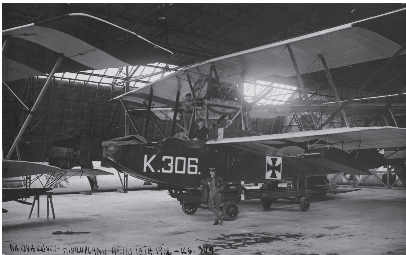
Proud airmen posing with Hansa Brandenburg W.13 K306 in Kumbor. The size of the aircraft and its 350 PS Daimler Ba. 21.000 engine is evident. White dots in its individual code identify this aircraft as being produced in Germany.
